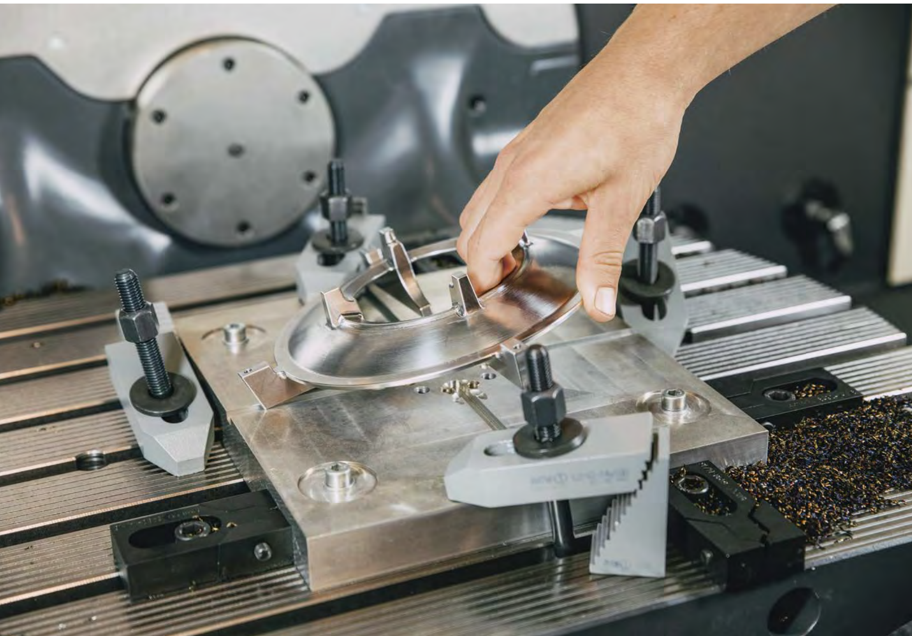
Left: To make the prototype a pan support is cut from a 5-cm-thick sheet of steel.
